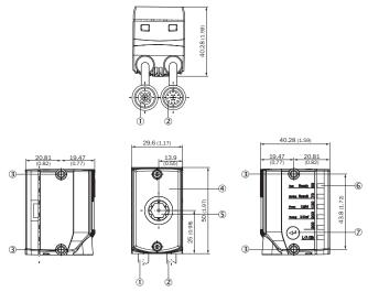
① Connecting cable with "Ethernet" connection (female connector, M12, 4-pin, D-coded), length of cable: 0.25 m
