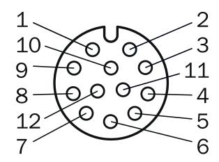
M12, 12-pin female connector, A-coded (I/O)
