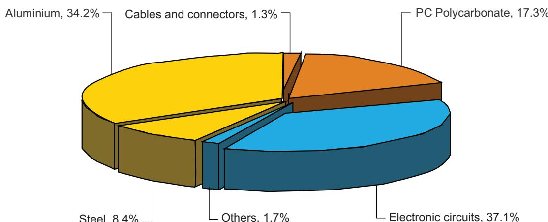
Products of this range are designed in conformity with the requirements of the RoHS directive (directive 2002/95/CE of 27 of January 2003) and do not contain, or in the authorised proportions, lead, mercury, cadmium, hexavalent chromium, flame retardant (polybromobiphenyles PBB, polybromodiphenylethers PBDE) as mentioned in the directive.
