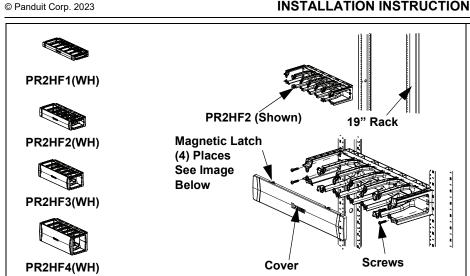
Install the managers to the rack with #12-24x1" screws provided. Install the cover to the manager by positioning the magnetic latches near the hinge pins of the manager. PR2HF1(WH) is installed with only 2 screws.
