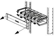
To open the cover downwards, pull out and down on the middle of the cover top. To open cover upwards, pull out and up on the middle of the cover bottom. To remove the cover completely, pull straight out on both ends of the cover simultaneously.
