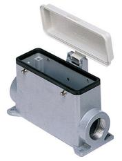
Surface mounting housing, C-TYPE series, with 4 pegs, Pg21 cable entry, size "104.27", with plastic cover
