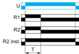
Function Hw: Interval Relay & with Retrigger / Restart Control
