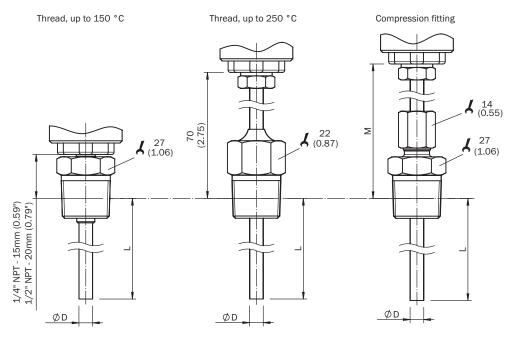
Dimensional drawing: housing, without process connection
