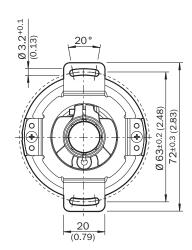
General tolerances according to DIN ISO 2768-mk  $\odot$  Cable diameter = 5.6 mm +/- 0.2 mm bend radius = 30 mm
