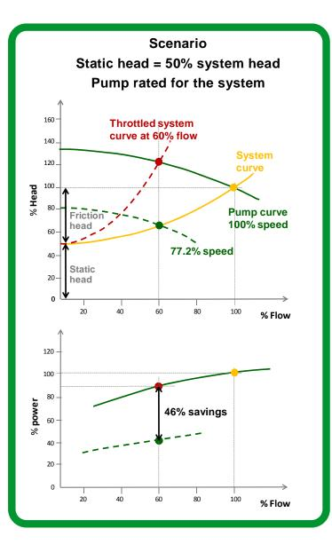
The example in **Figure 1** compares two installations (one with a variable speed drive one with a fixed drive throttled system) in which static heads (height difference between the source and the end use) are different.
