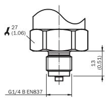
Housing with L-connector (DIN 175301-803 A), IP65
