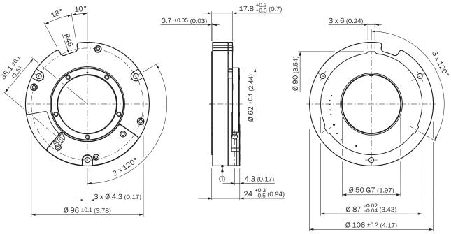
① Measuring point for operating temperature
