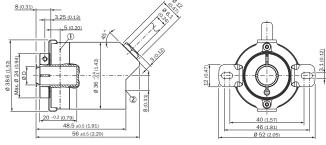
Non-tolerated dimensions according to DIN-ISO 2768-mk
