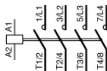
3-Pole Contactors: 3P + N/C
