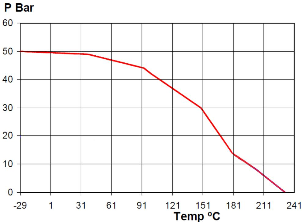
**ROBINET A TOURNANT SPHERIQUE 2 PIECES ACIER A BRIDES CLASS 300 PN50 ICP**
