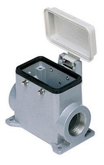
Surface mounting housing, C-TYPE series, with 4 pegs, Pg21 cable entry, size "57.27", high construction, with plastic cover
