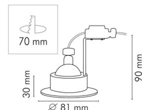
SPOT IP44 max 35W max 50W 850°C IP44 MAX 50W
