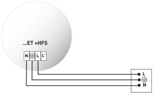
To switch further luminaires via the sensor luminaire, a power contactor is installed over the switching output (L').
