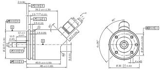
Non-tolerated dimensions according to DIN-ISO 2768-mk
