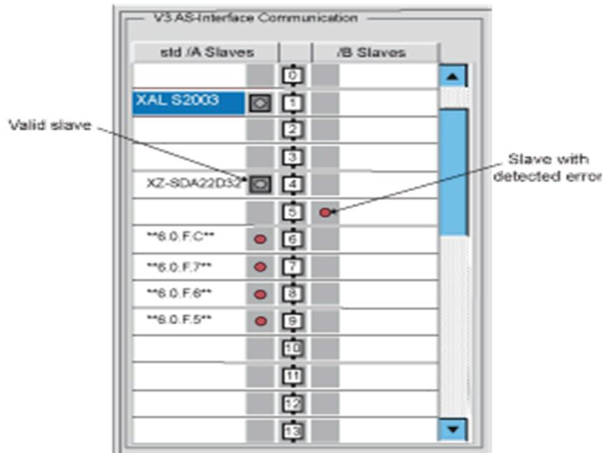
**NOTE:** As 6.0.F.C above shows, when there is a detected error on a slave with a S-6.0 profile, all of its virtual “slaves” are also indicated to have detected errors.
