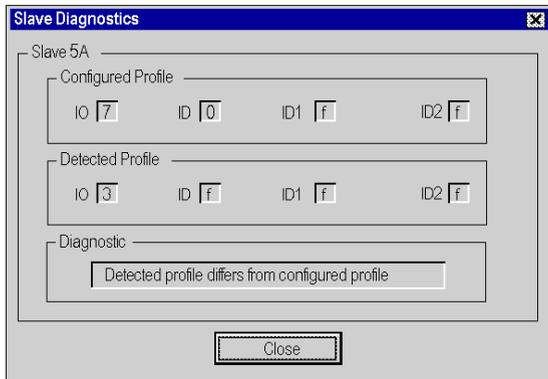
This window displays the following detected errors for each slave device:
