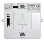
Device that enables regenerating the Duox signal in both directions, isolating different sections of the installation and expanding terminal distances and capacities. Inputs and outputs get isolated as protection against short circuits, load and signal reflections.
