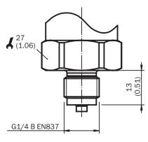
Housing with L-connector (DIN 175301-803 A), IP65
