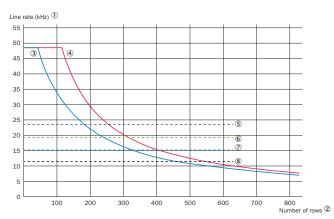
The maximum line rate is based on the number of sensor lines used
