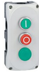
Grey control station LPZP3A8 complete with green flush pushbutton "i" LPCB1113 1NO, red extended pushbutton "o" LPCB2104 1NC and green pilot light 24V LPZP3B8911
