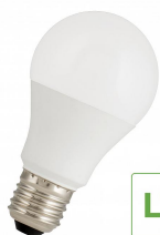
80100040597 LED A60 E27 24V AC/DC 7W (60W) 800lm 827
