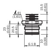
Housing with L-connector (DIN EN 175301-803 A)
