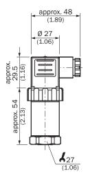
Process connection with flush-mounted membrane, G 1 B with/without cooling element, 0 ... 0.1 up to 0 ... 1.6 bar
