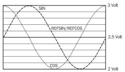
Signal diagram for clockwise rotation of the shaft looking in direction "A" (see dimensional drawing)1 period =  $360 \degree : 1024$
