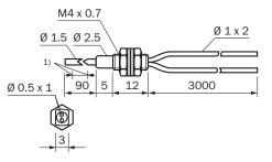
Flexible end tip, do not bend in this area (10 mm), bend radius R10 mm
