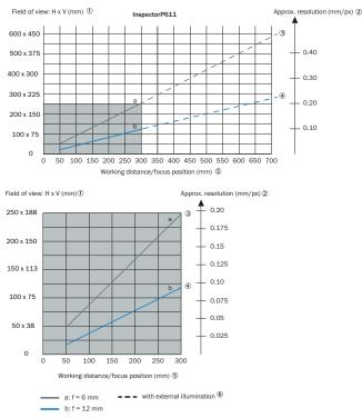
Take into account the following aspects when designing the application: the field of view geometry of the device, and the position of the field of view in the space in front of the device. Possible angles at which the objects can arise in relation to the device. For the planned working distance: resultant field of view length and width as well as the approximate resolution.
