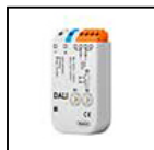
S.2492 Signal converter from DALI to VIRTUAL MIDNIGHT. Compact control IP20 module for automatic power reduction / brightness reduction for night-time. The device has an integrated bus supply (20mA) for up to 7 DALI luminaires. Possibility to extend up to max. 64 luminaires through the DALI Expander (S.2494). 2 operating modes are supported: - Operating mode B1: power reduction through mains phase or control phase; - Operating mode B2: power reduction using virtual midnight calculation. All necessary settings can be made using rotary and slide switches. The device must be located before the DALI luminaire inside an electrical cabinet / waterbox / junction box.
