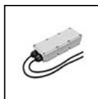
S.2497 Signal converter from DALI to VIRTUAL MIDNIGHT (max 64 luminaires) Compact control module for automatic power reduction / brightness reduction for night-time. The box has a converter from DALI to VIRTUAL MIDNIGHT device and DALI EXPANDER (200mA) device integrated, that allows to control up to 64 DALI luminaires / DALI control gears within 300 meters. 2 operating modes are supported: - Operating mode B1: power reduction through mains phase or control phase; - Operating mode B2: power reduction using virtual midnight calculation. All necessary settings can be made using rotary and slide switches present on the device present inside the waterbox. The device must be located before the DALI luminaire / DALI control gears.
