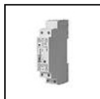
S.2494 DALI EXPANDER The IP20 DINrail device is used to extend a DALI circuit via broadcast. The received input signal is amplified and transmitted in broadcast to the DALI luminaires / DALI control gears. The DALI Expander has an integrated DALI bus power supply (200mA) which can control up to a maximum of 64 DALI devices within 300 meters.
