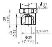
Housing with L-connector (DIN 175301-803 A), IP65
