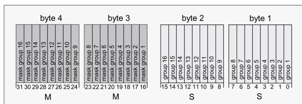
Figure 13: Structure of the objects of the collective feedback, using the example of the object for Groups 1-16
