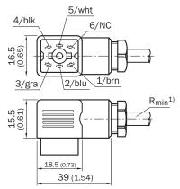
(1) Minimum bend radius at dynamic use  $\rm R_{min}$  = 20 x cable diameter
