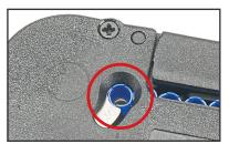
Ensure that first ferrule is seated into the die pocket as shown above.
