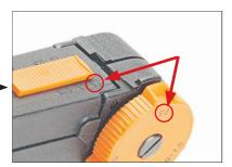
Press in and rotate adjustment dial, until desired die setting is reached. Adjustment dial will automatically click into place when setting is reached. Adjust slide control on cover so that the two settings match. These two settings must match to crimp correctly.
