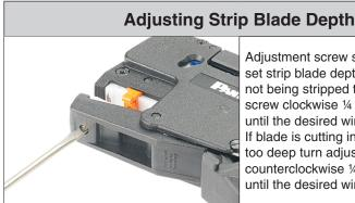
Adjustment screw should be used to set strip blade depth. If insulation is not being stripped turn adjustment screw clockwise 1/4 turn increments until the desired wire strip is achieved. If blade is cutting into insulation too deep turn adjustment screw counterclockwise 1/4 turn increments until the desired wire strip is achieved.
