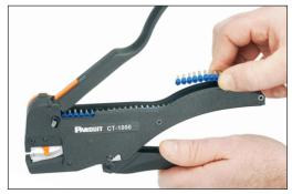
Close the cover. If the end of the ferrule strip is longer than the handle (as shown above), fold over and close cover.
