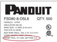
With door open, make dial and slide adjustments to match specific setting noted on package label.
