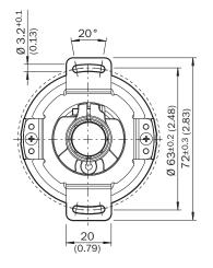
General tolerances according to DIN ISO 2768-mk (1) Cable diameter = 5.6 mm +/- 0.2 mm bend radius = 30 mm
