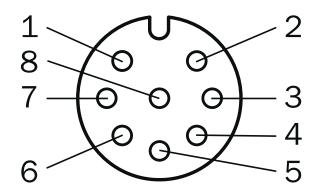
Female connector M12, 8-pin, A-coded
