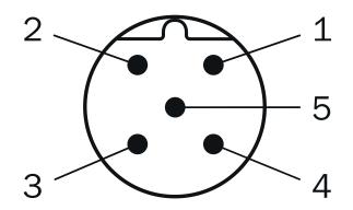
Male connector M12, 5-pin, A-coded
