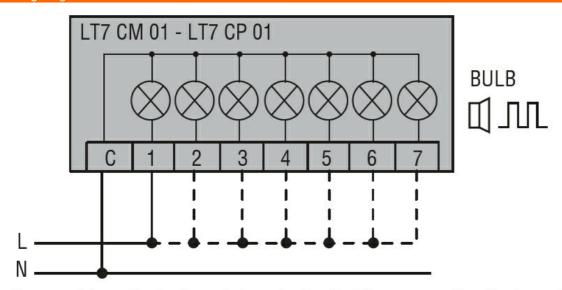
Connect terminals C and 1 as indicated to power the first module. If other modules are fitted, the respective terminals must be connected accordingly.
