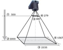
Fig. 9: Field of view V2D8512R-xxxxxxx, focal length: 16 mm
