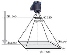
Fig. 10: Field of view V2D8512R-xxxxxxx, focal length: 25 mm
