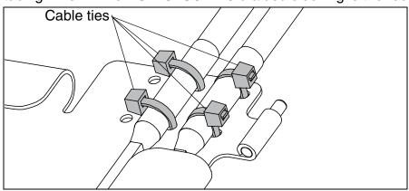
Using cable ties, secure the fiber to the splice tray as shown.
