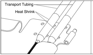
It is recommended that transport tubing is used to keep the buffer tubes bundled. Cut 2" sections of heat shrink tubing. Heat shrink the heat shrink tubing over the exposed buffer tubes and transport tubing to secure the fiber to the transport tubing. The *PANDUIT* SE25PSC-TR0 braided sleeving is the recommended transport tubing.
