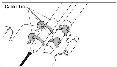
Using cable ties, secure the fiber to the splice tray as shown.
