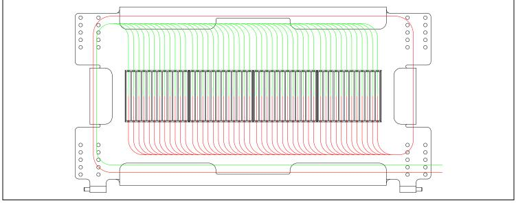
Route the fiber as shown in the image. Splice protectors as well as heat shrink tubing and transport tubing, as describer earlier, should be placed over fiber prior to splicing.
