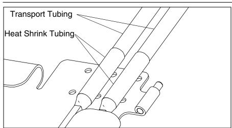
Cut 2" sections of heat shrink tubing. Heat shrink the heat shrink tubing over the grommet, part of the exposed ribbon (on the tray side of the grommet) and transport tubing to secure the fiber to the transport tubing. The *PANDUIT* SE25PSC-TR0 braided sleeving is the recommended transport tubing.
