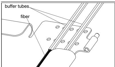
The incoming and outgoing fiber should be grouped together as shown. The buffer tubes will be secured directly to the tray and should be positioned over the cable tie holes as shown. The grommets are not required in this arrangement.
