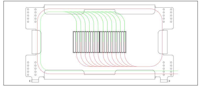
Route the fiber as shown in the image. For 12 fiber ribbon, install splice protector in every other mounting groove of the splice holder. Splice protectors as well as heat shrink tubing and transport tubing, as described later, should be placed over the fiber prior to splicing.
