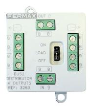
The BUS-2 distributor is a device which is responsible for routing the bus from the panel to the active monitor/telephone, maintaining the power supply and the data signal on all monitors/telephones at all time. Only for installations with b/w monitors.The distributor opens the path to the active monitor/ telephone and prevents video and audio signals reaching the rest of the branches.
