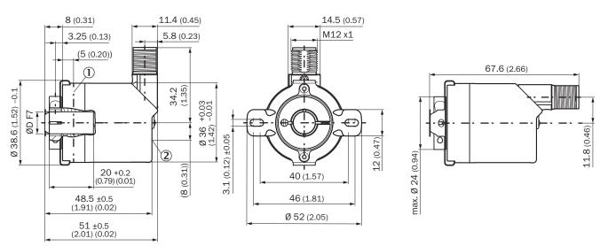
① Measuring point for operating temperature
