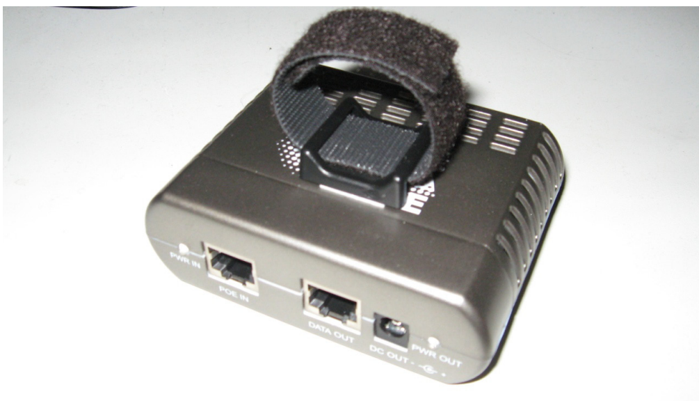
Figure B - Hook and loop strip attached to power splitter
