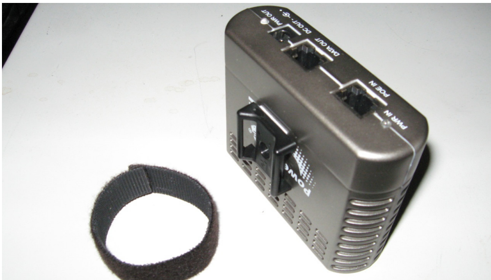
Figure A - Hook tie mount attached to power splitter
