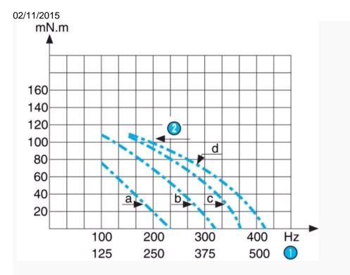
Inertia of measuring chain : 3.4 g.cm2 a = constant voltage controller with Rs (resistance in series) = 0 b = constant voltage controller with Rs (resistance in series) = R motor c = constant voltage controller with Rs (resistance in series) = 3R motor The measurements are made with full stepping, 2-phases energised.
