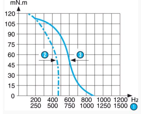
Inertia of measuring chain : 3.4 g.cm2 a = constant voltage controller with Rs (resistance in series) = 0 b = constant voltage controller with Rs (resistance in series) = R motor c = constant voltage controller with Rs (resistance in series) = 3R motor The measurements are made with full stepping, 2-phases energised.
