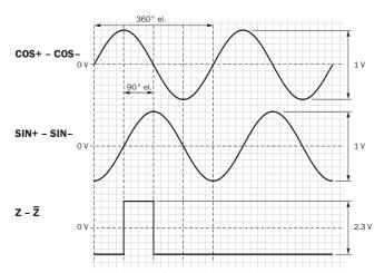
For clockwise shaft rotation, looking in direction "A" (see dimensional drawing) Maximum revolution range
