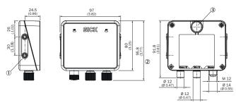
Structure and device dimensions, unit: mm (inch), decimal separator: period
