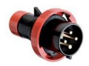
Mobile plug, PLUSO HEAVY DUTY series, 3 poles + N + PE, 6 h (red), 32 A,  $380 \div 415 \text{ V}$ , straight
