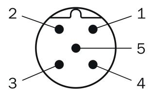
Male connector M12, 5-pin, A-coded
