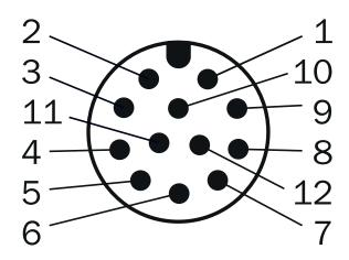
M12, 12-pin male connector, A-coded
