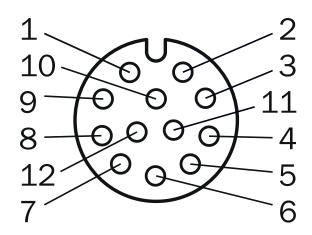
M12, 12-pin female connector, A-coded (I/O)  $\,$
