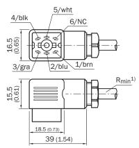
$\bigcirc$  Minimum bend radius at dynamic use R<sub>min</sub> = 20 x cable diameter
