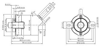
Non-tolerated dimensions according to DIN-ISO 2768-mk
