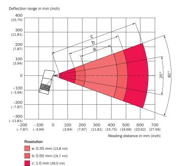
① Diagram applies to focus position of 280 mm
