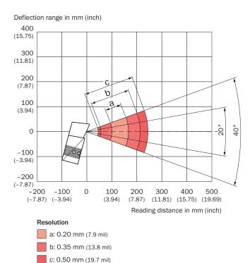
① Diagram applies to focus position of 140 mm
